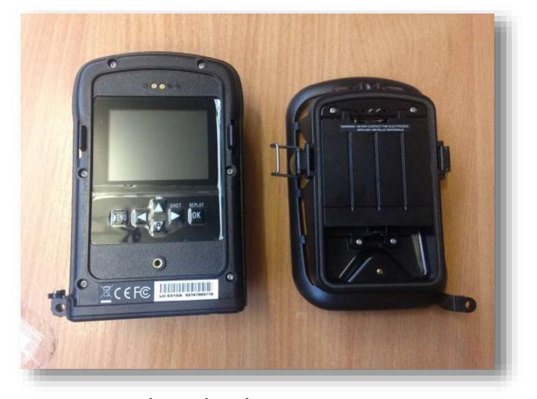
Undo side clips to open camera trap
